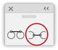
**'C':** [When drawing multi-lines] Toggles between Offset and Centring the lines
