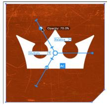
When holding the SHIFT key down and clicking on the rotation annotation control, the rotation changes in 45 degree increments
